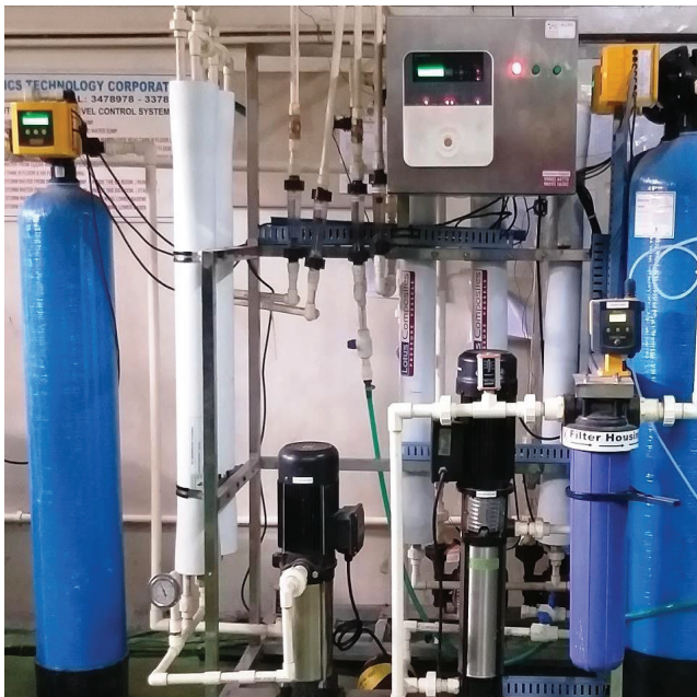
In house Ro Plant and unique steel bubble top dispensers designed by Sasken
